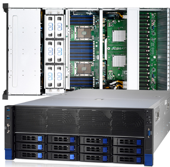
Figure 1: Thunder HX FT83-B7119 - 10-GPU Server Platform for HPC/AI/ML/DNN Workloads
