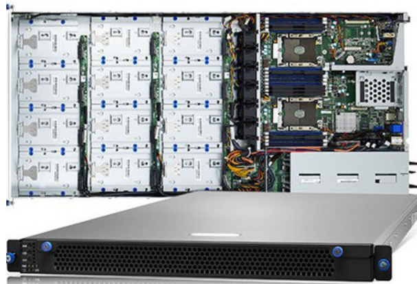
Figure 2: Thunder SX GT93-B7106 - 1U Density Storage Server with 12 Internal 3.5" SATA 6G Drive Bays and dual socket Intel Xeon Scalable Processor
