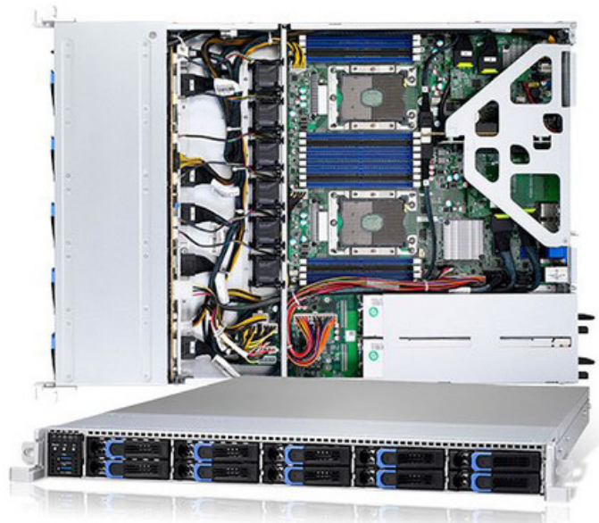
Figure 1: Thunder SX GT62H-B7106 - 1U All-Flash Dual Socket Storage Server
